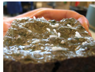
Alkali-silica gel extruded from reacted concrete. Courtesy of Jan Lindgård.
