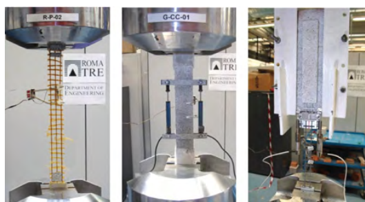
Testing setup for the round robin tests on mortar based composites. Courtesy of Gianmarco de Felice.
