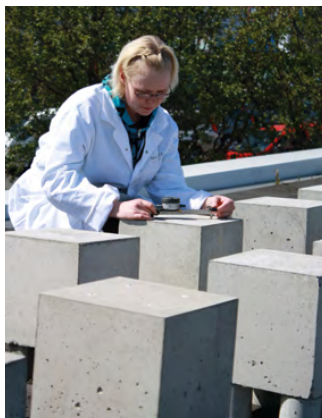
Expansion measurement at an outdoor exposure site. Courtesy of Børge Johannes Wigum.
