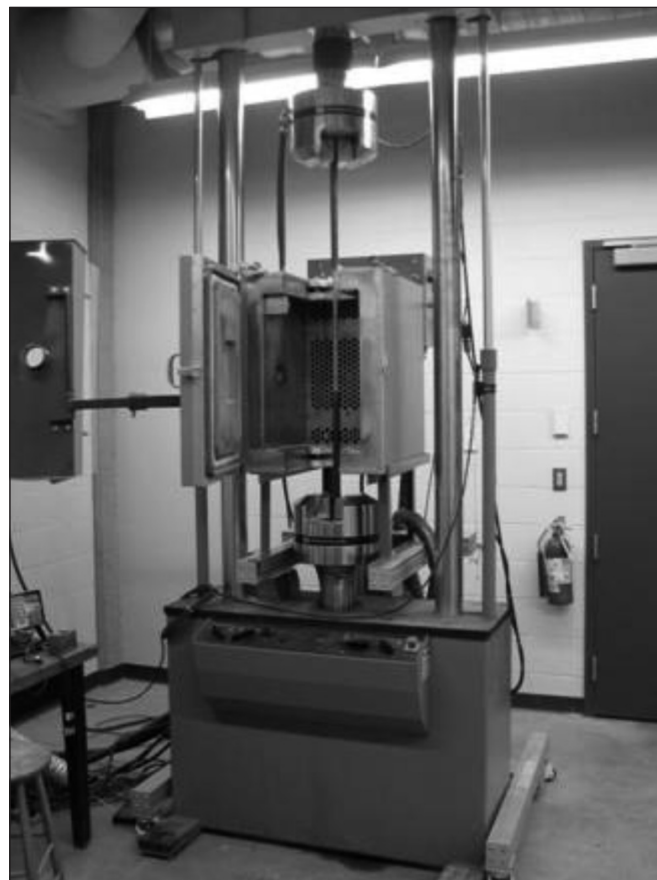
Figure 4: Test setup for tensile tests at controlled temperature
