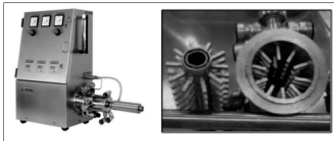
Figure 3: Example of an industrial foam gun (stator and rotor details).
