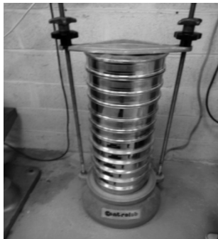
Figure 4. Essai de tamisage.
