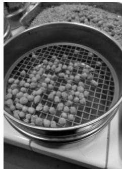
Figure 4. Essai de tamisage.
