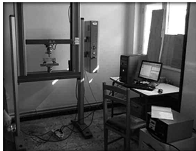
Figure 2. Machine universelle type Zwick/Roell, capacité 20 KN
