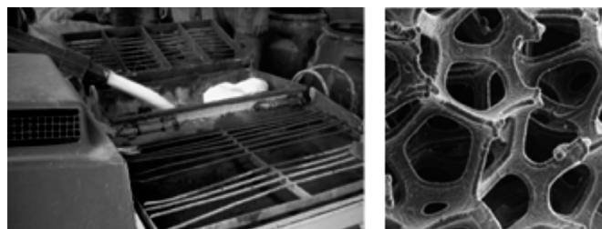
Figure 4: left: Adding foam in the gauging chamber of a mixer. Right: Foam deposit on a metal substrate (www.recemat.nl).
